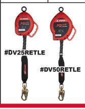
KStrong® BRUTE™ 25' - 50' Galvanized Wire Cable SRL-LE (ANSI Leading Edge Rated) with High Impact Strength Polymer Housing with Built-in Handle, swivel eye at anchorage end, other end with load indicator swivel snap hook.
