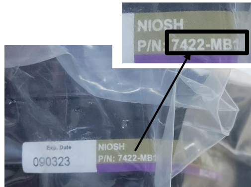
Cartridge incorrectly labeled as 7422-MB1
